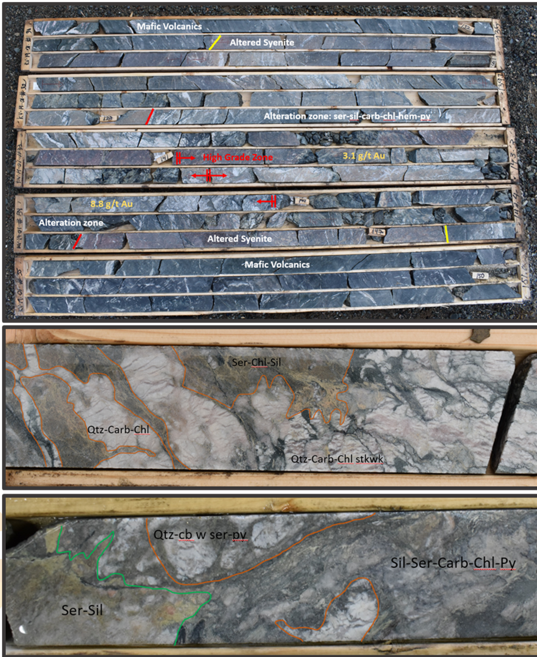
Figure 4. Core photos of KV-19-01 exhibiting the intensely altered contact of the volcanics and syenite associated with gold mineralization.
