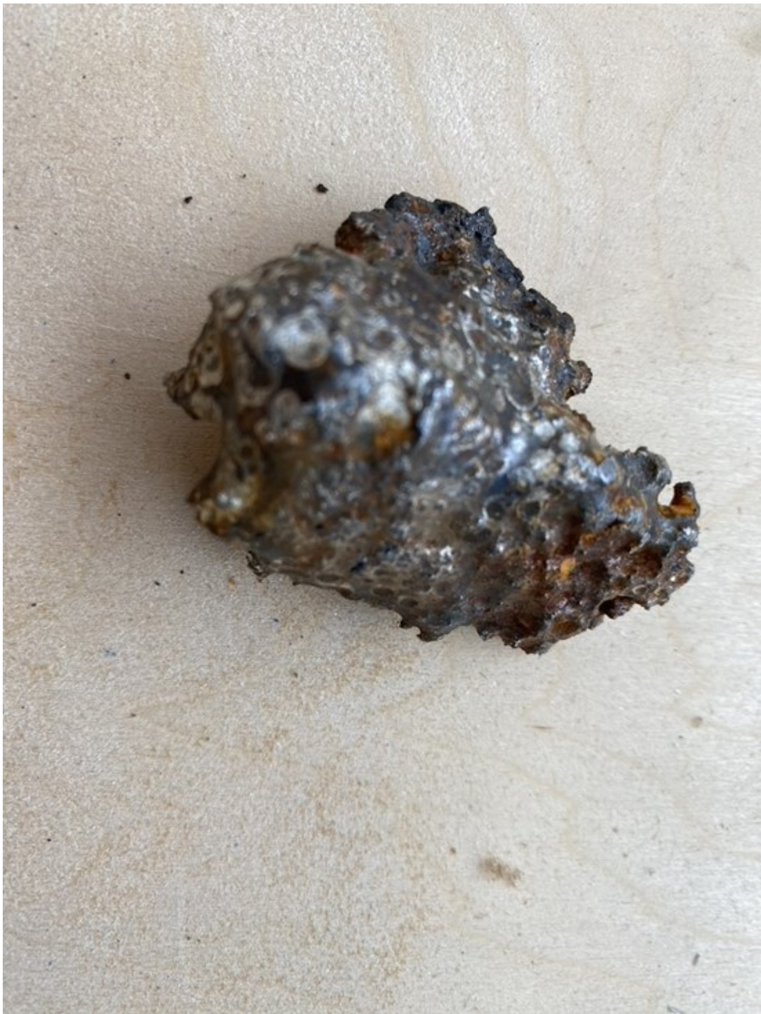
Malformed refractory dore bar poured in September, 2022
