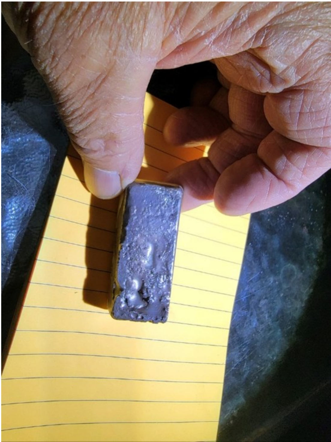
Dore bar poured after the iron alloy was removed; Feb 2023
