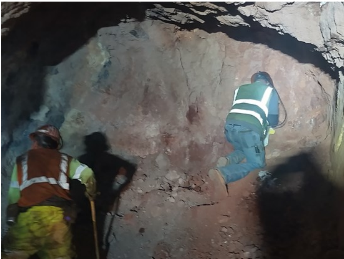
Sawing channel sample across the face of the vein at 444ft from the portal entrance, late February, 2023
