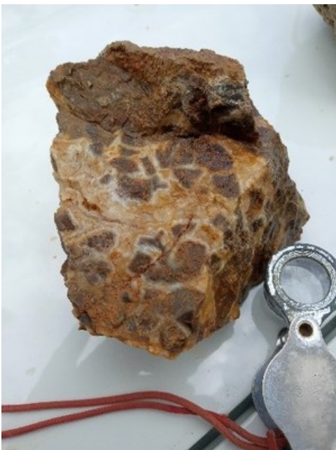
Figure 5: Quartz-sulphide vein and colloform banded quartz matrix breccia float from Kerefa Prospect (CNW Group/Kainantu Resources Ltd.)
