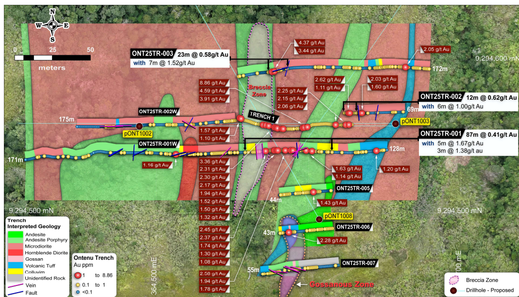
Figure 10 Ontenu Central (westside corridor) trenching
