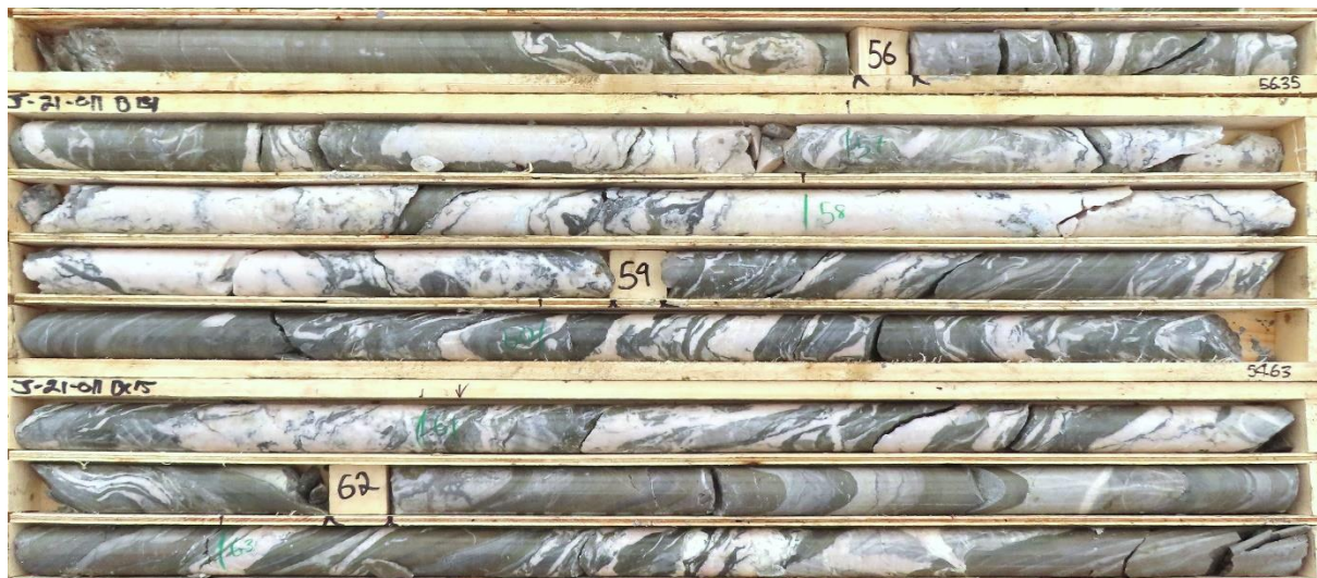
Figure 4 – Quartz flooding with abundant arsenopyrite in patches, veinlets and stylolites, from roughly 56 m to 62 m downhole in J-21-011. Assays for this and other mineralized zones in J-21-011 are pending.
