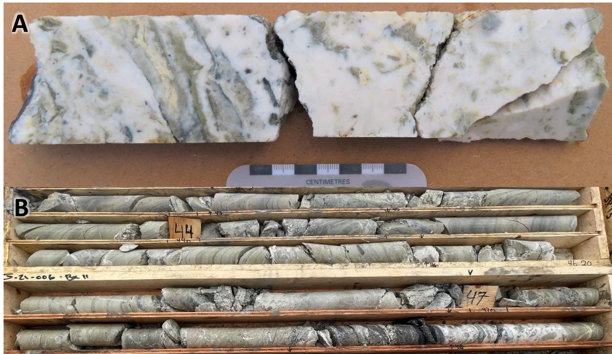
Figure 2 A) Quartz-carbonate vein material from drill hole J-21-006 (47.98 to 48.23 m downhole), as shown in previous SGD exploration release dated July 14, 2021. This quartz vein and the preceding fault zone returned 10.65 g/t Au across 0.7 m, at the base of a mineralized interval.
