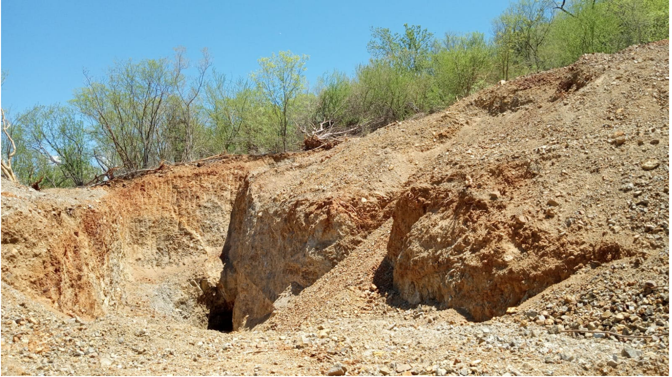
Photo 3. Active trenching of at surface oxide gold-silver material across expansion targets.
