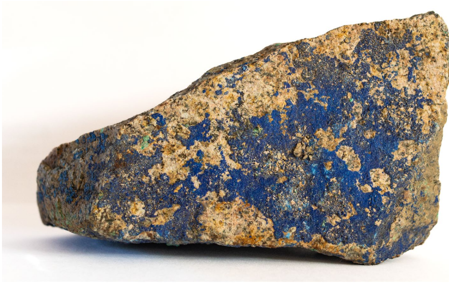
Figure 3-Azurite and malachite mineralization in lower trench beside collar of S-061 as 20 cm long angular subcrop. Star Copper 2025.
