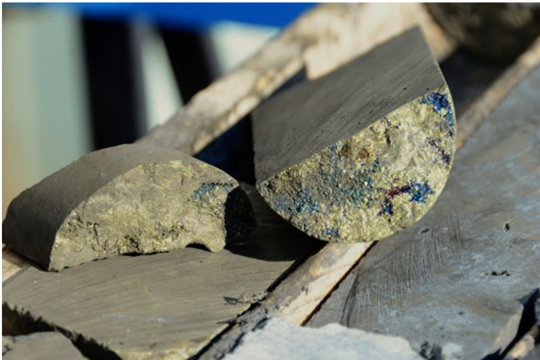
FIGURE 4: Chalcopyrite and Covellite, (140.45m.) - Horizon 1
