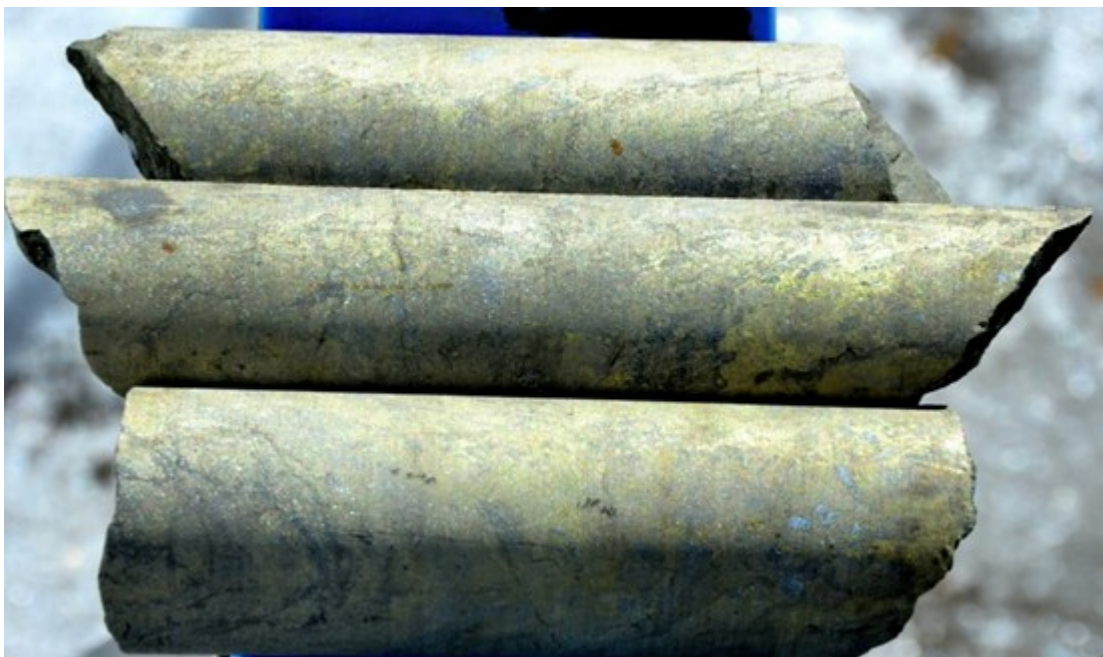
FIGURE 5: Semi Massive Chalcopyrite, Sample 338291 (6.52% Cu) - Horizon 2
