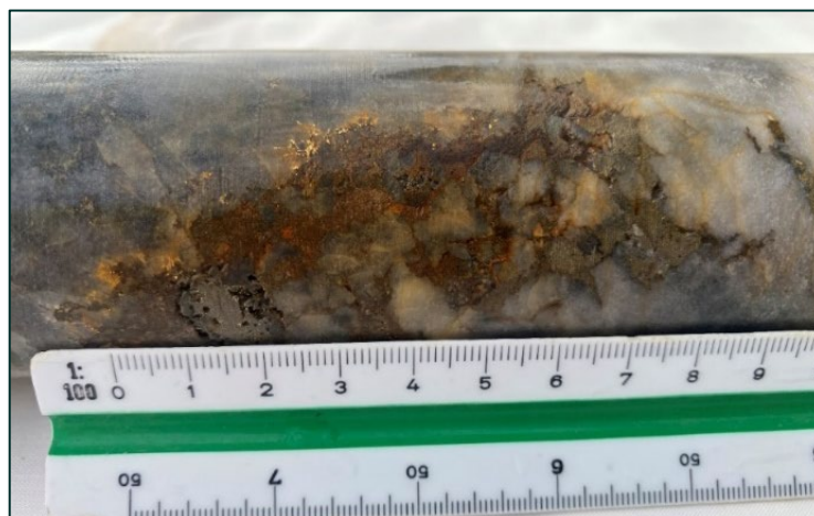
Figure 1 - 24GFDD022 visible gold at 204.87m associated with quartz veining.
