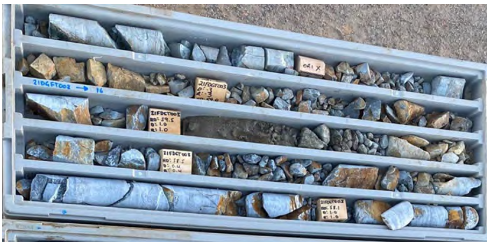
Figure 16-13 ‘Sand Zone’ intersected in hole 21FDGT003. Source: Westgold.
