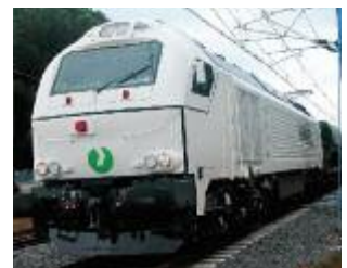
EURODual—also runs on trackage with overhead wires
