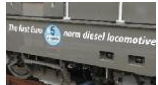
G 6 ME—the first shunting locomotive to meet the Euro 5 emissions norm
