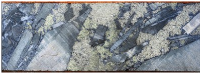
Figure 4: Typical breccia mineralisation: angular silica-tourmaline altered siltstone clasts supported in a pyrite- chalcopyrite-tourmaline-quartz matrix. The breccia matrix at San Francisco is sulphide-rich, with 60-90% sulphides by volume. SFDH-002, 108m. From a 1m sample that averaged 3.5 g/t gold, 36 g/t silver and 1.1% copper. (CNW Group/Turmalina Metals Corp.)
