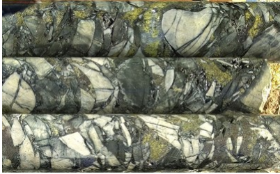
Figure 2: Typical gold-silver-copper-lead-zinc breccia mineralisation: sericite-silica-tourmaline altered clasts of quartzite and siltstone set in a chalcopyrite-pyrite-sphalerite-quartz-tourmaline matrix. (CNW Group/Turmalina Metals Corp.)
