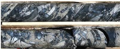
Figure 3: Typical gold-bearing breccia mineralisation: angular sericite-silica altered clasts of quartzite and siltstone set in a pyrite-tourmaline-quartz-chalcopyrite matrix. SFDH-002, 75-76m; from a 2 m interval that averaged 5.6 g/t gold, 244 g/t silver & 0.37 % copper. (CNW Group/Turmalina Metals Corp.)
