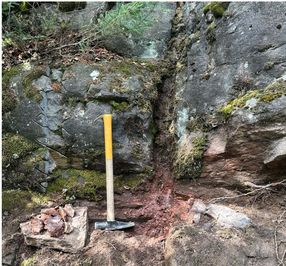
Figure 9-17. Fault-Controlled Mineralization and Alteration at the Manhattan Showing, Reaching >65,535 cps on the handheld RS-125
