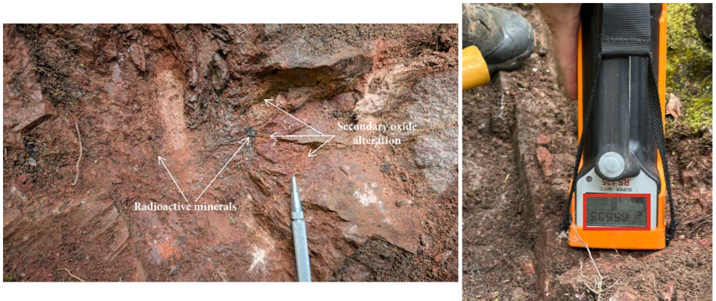
Figure 9-16. (Left) Close-up of Fault-Controlled Mineralization (black vitreous minerals) (Right) Iron Oxide Alteration on Surface at the Manhattan Showing (Dorward Lake area), Reaching >65,535 cps on the RS-125
