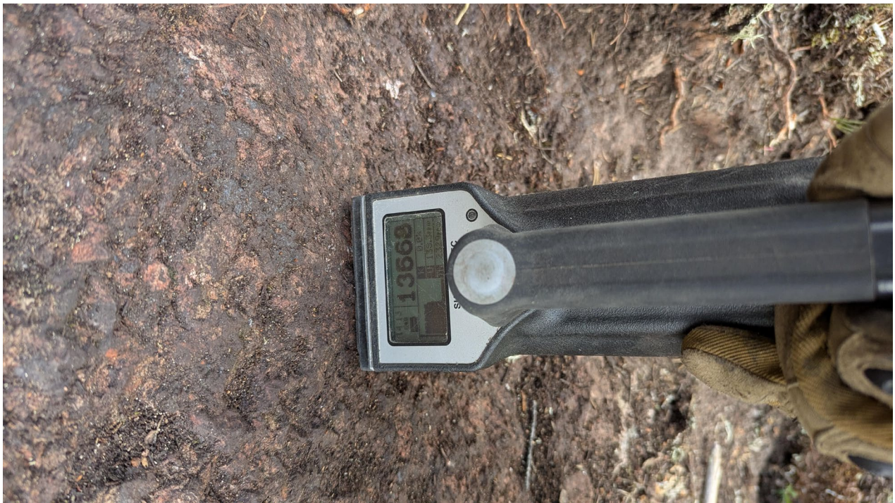
Figure 9-15. Hematized Magnetite-rich Pegmatite at the RANEZ Showing North of T-Lake; Maximum of >13,500 cps on the RS-125 Super-spectrometer
