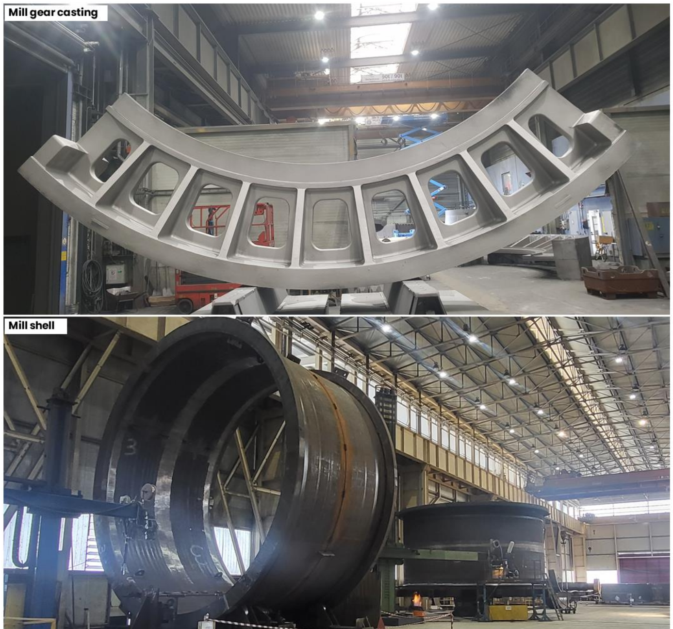
Figure 2: Mill gear casting and shell being fabricated
