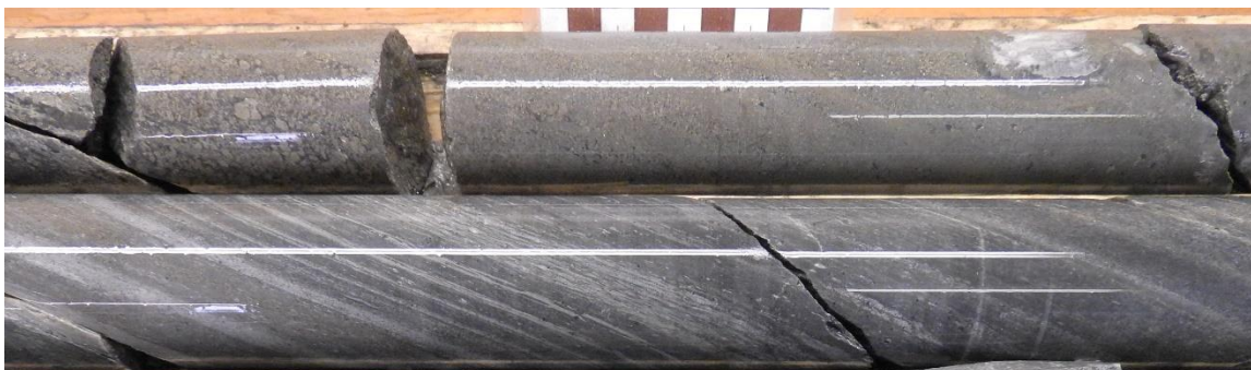
Figure 7-39 Felsic Tuff with Lapilli and Quartz Crystals, Containing Beds and Laminations of Massive Pyrite and Locally Laminations of Sphalerite, Drill Hole 1274-16-226 at 628 m
