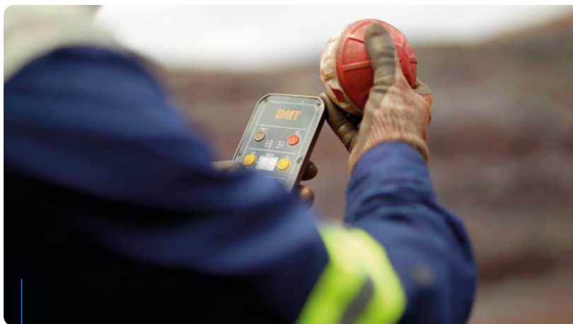
Field technician Johan Burden activates a blast movement monitor before inserting it into a drillhole to track the movement of the ore following a blast.
