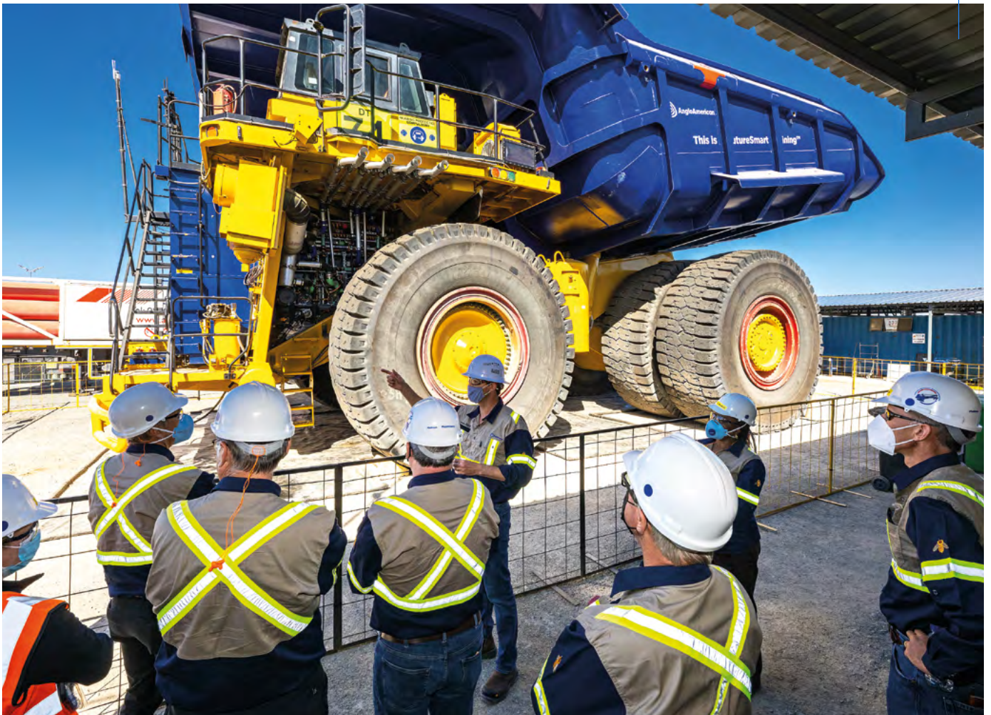
At Mogalakwena in June, Board members and executives are briefed on the prototype nuGen™ hybrid hydrogen and battery powered heavy haul truck, which was officially launched at the mine the previous month.
