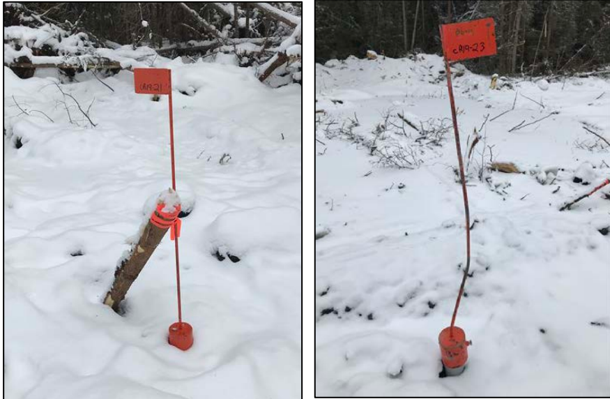
Photo 5. All drill casings have been left in place. The casings are routinely capped and marked by metal flags for future reference. Drill holes CR19-21 and CR19-23 are presented here (CR19-14a in the previous photo).
