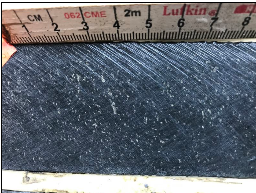
Photo 17. Close-up view of a section of the core included in the previous photo. Disseminated sulphides and awaruite (NiFe alloy) are present in the core included in sample 966932 from 372 m to 373.5 m in drill hole CR19-14a.
