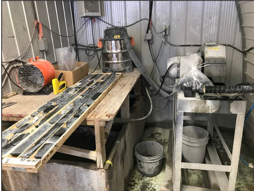
Photo 15. Diamond-blade core saw for cutting the half drill-core samples that are submitted for analysis. The separate cutting room is isolated from the logging area and located at the front corner of the building. A second saw in the room is also available for sampling use.
