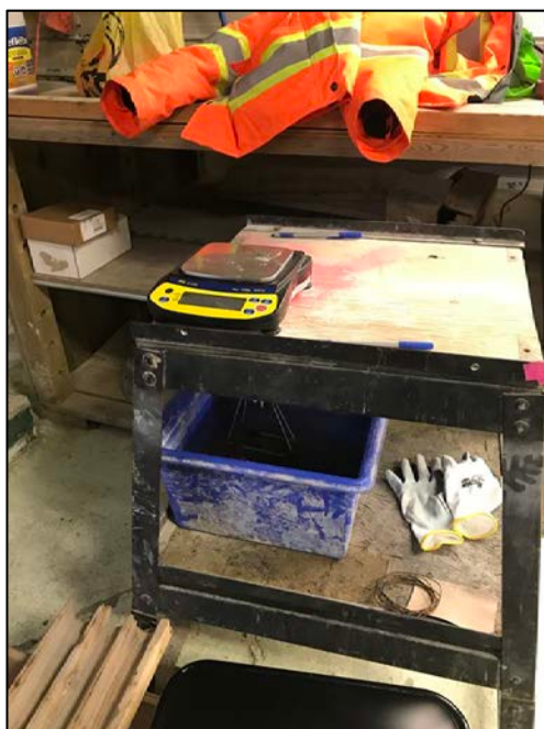
Photo 14. Weigh scale set-up for the field determination of the relative density ("SG") of selected samples using wet vs. dry weights.
