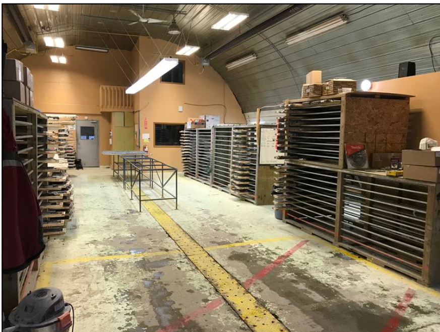
Photo 10. Indoor storage racks are used to hold the drill core while it is actively being logged and sampled (and being thawed in winter). Logging benches are located to the left and right of the photo behind the storage racks.
