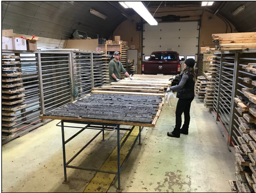
Photo 11. Core boxes brought in from the field being unloaded from a pick-up truck. Boxes are opened and prepared (i.e. the core is measured and marked) in this area prior to logging.
