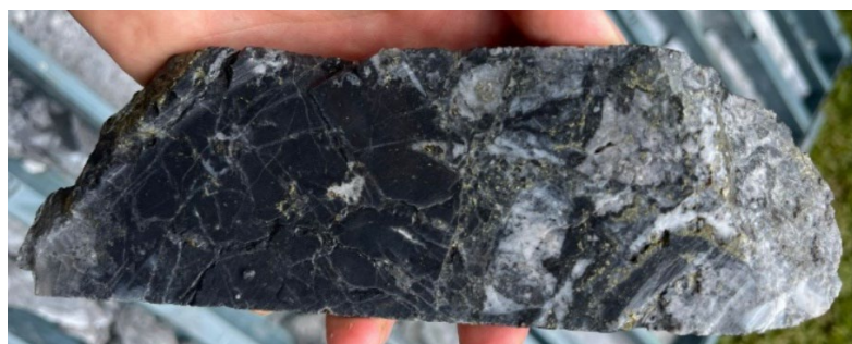
Figure 3: HQ drill core specimen from WDG-12 (181m) showing a dark grey to black clast-supported hydrothermal breccia cemented by chalcopyrite, pyrite, and quartz.
