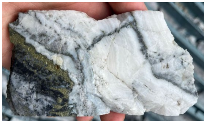
Figure 4: HQ drill core hand specimen from WDG-12 (179.6m) showing massive quartz–carbonate–sulphide veining with coarse chalcopyrite and pyrite, typical of a strongly mineralized vein zone within the Sinivit system.
