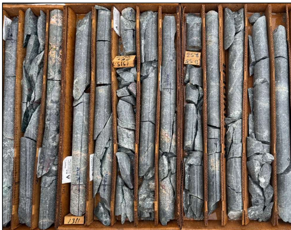
Fig. 4a. Bilk intrusion with potassic alteration from hole SK-26-07, 1,309-1,329'.
