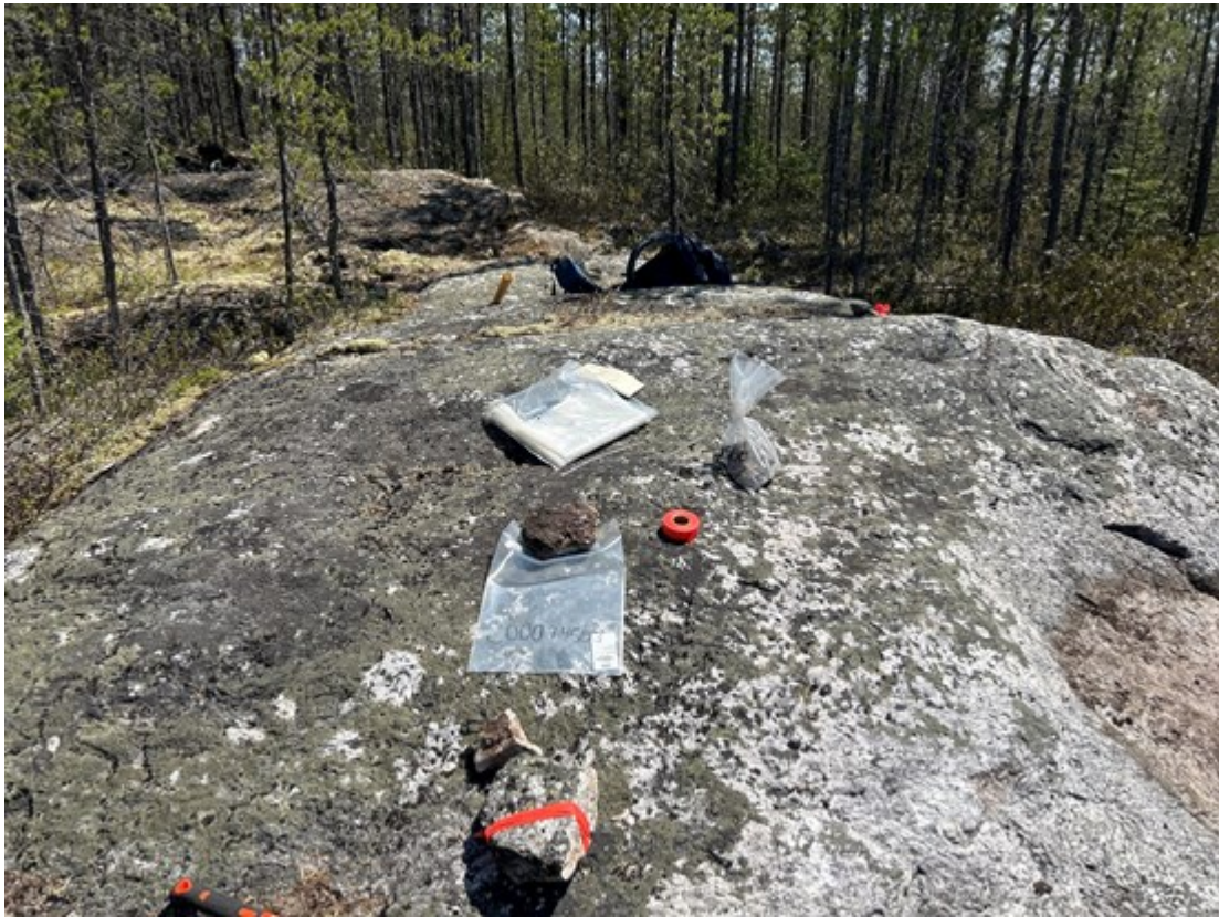
Figure 3: Chou Showing outcrop with three samples that returned >1.17% to 2.33% Li 2 O
