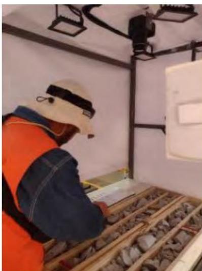
Figure 8.1: Dedicated static photo booth for consistent photography of core
