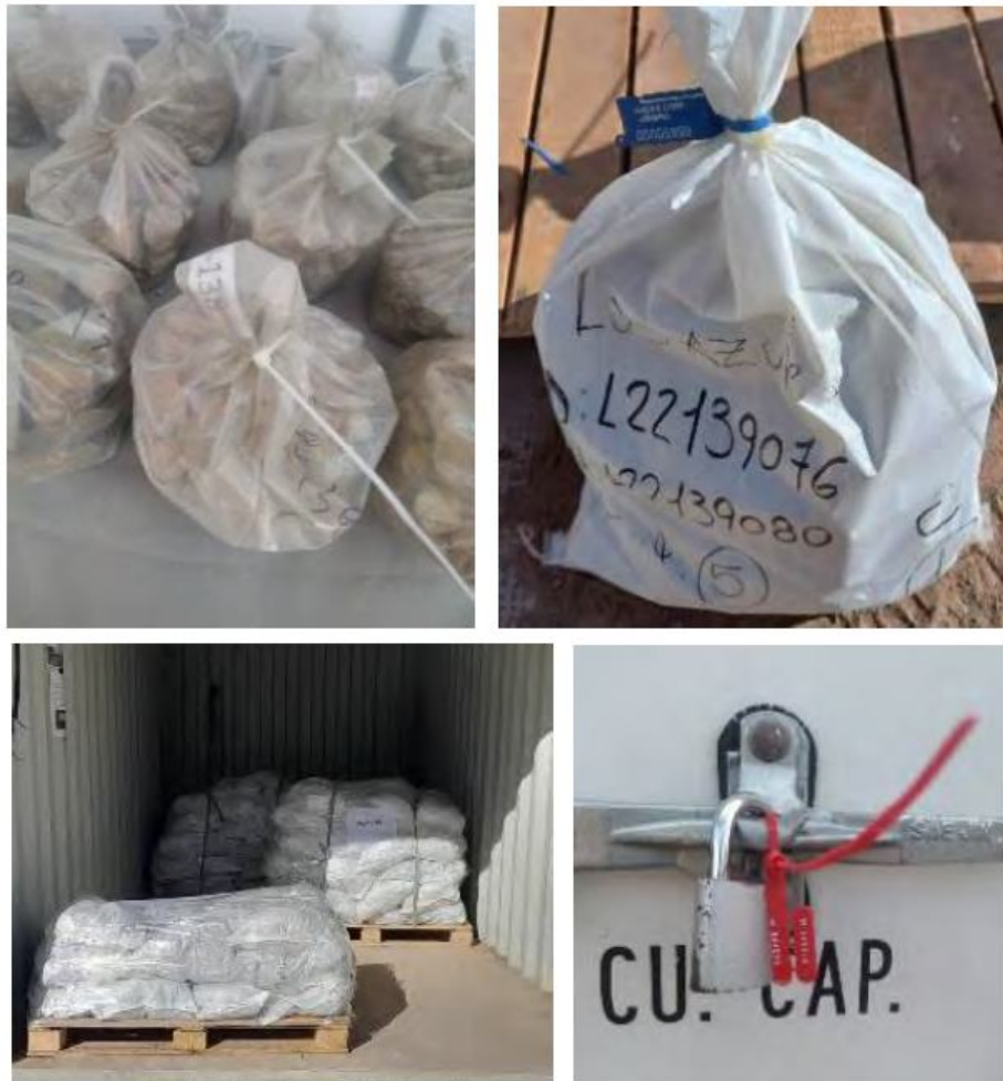
Figure 8.5: Showing the sequence of bagging, tagging, sealing, and securing the samples for dispatch.
