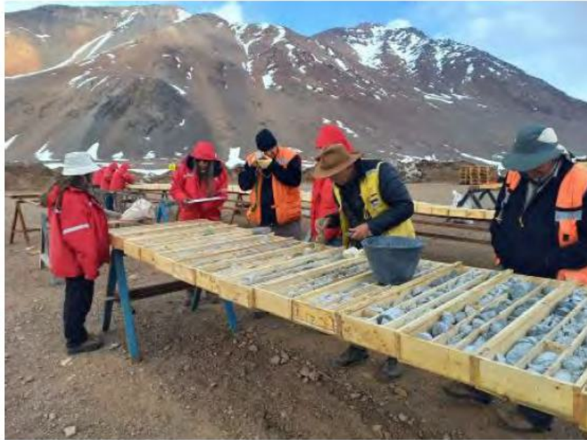
Figure 7.5: Logging and inspection of drill core
