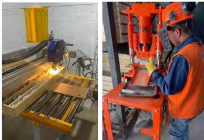
Figure 8.4: The hyperspectral scanning unit and the hydraulic core splitter
