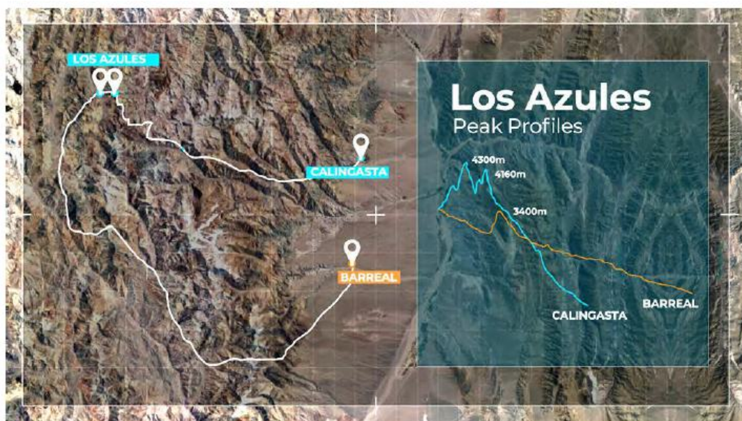
Figure 15.4: Site Access Road Profiles (McEwen)
