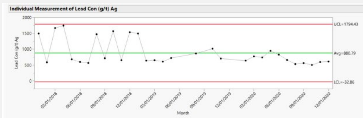
Figure 13-5: Toll Treatment Lead Concentrate Ag Grade Control Chart
