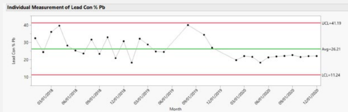
Figure 13-4: Toll Treatment Lead Con. Pb Grade Control Chart
