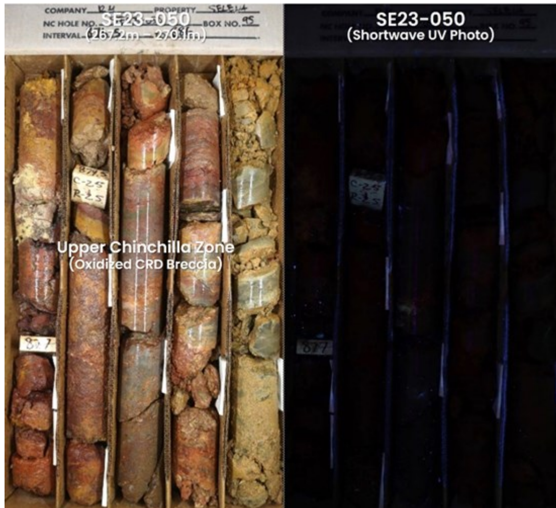
Picture 2 : Representative core and shortwave UV photo of the Upper Chinchilla Zone SE23-050. Note the lack of "BBQ Rock" fugitive calcite veins, which typically occur on the margins of the CRD system
