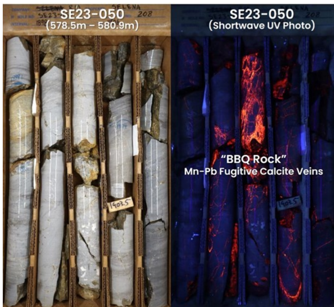
Picture 3 : Core and Shortwave UV photo of "BBQ Rock" (fugitive calcite veins) at depth in SE23-050.
