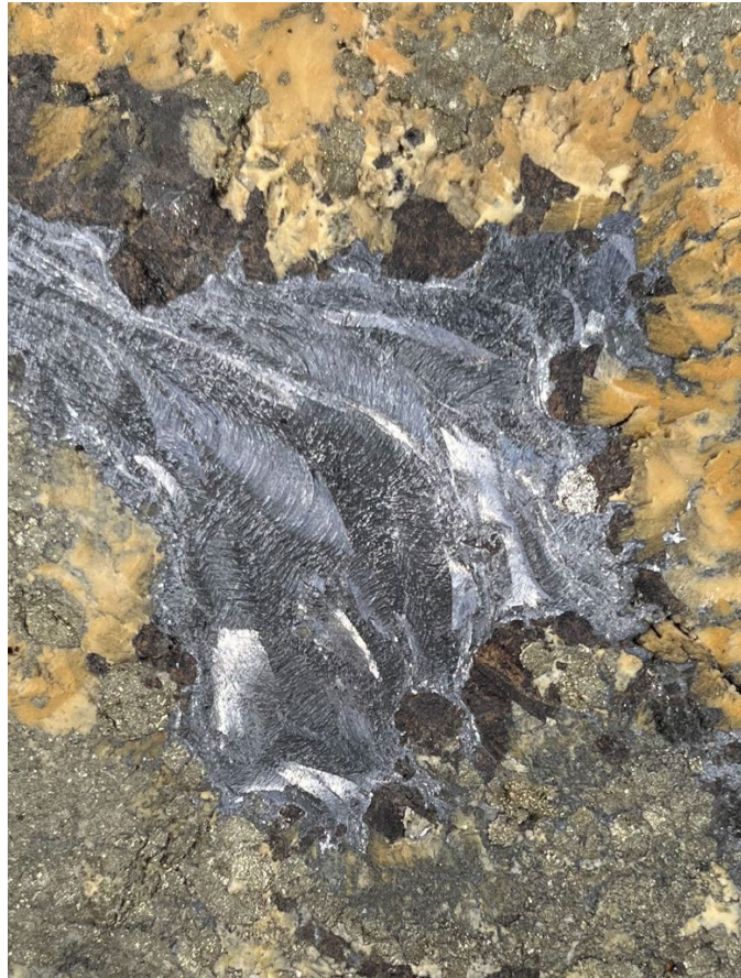
Figure 7.10: Argentiferous Galena with Pyrite, Fe-Rich Sphalerite and Dolomite
