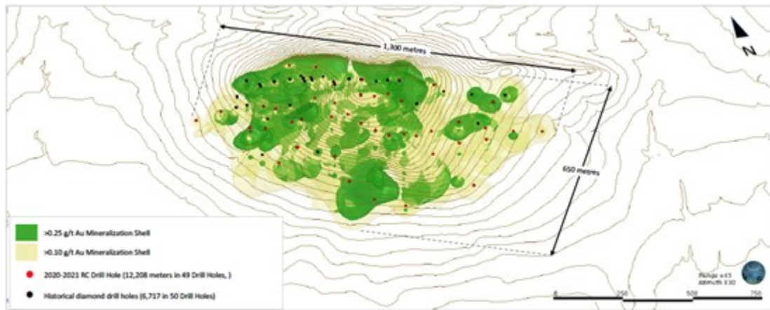
Figure 3b: Expansion of mineralization at the Capitan Hill oxide-gold deposit (3D View)
