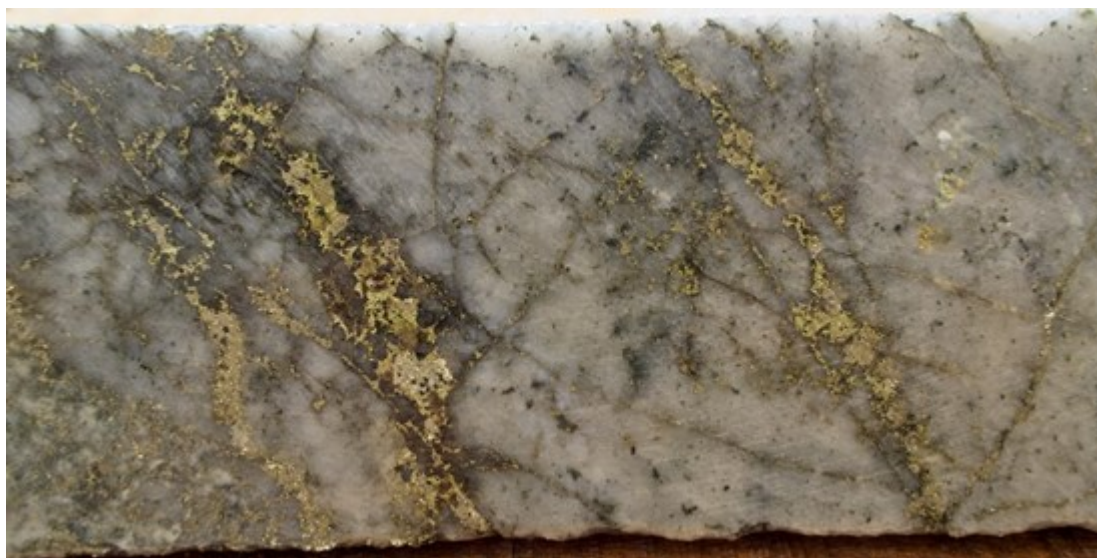
Image 2. ELID023, 397.5 m from a 2 m long sample interval reporting 1.07% Cu, 0.003% Mo, 14.6 g/t Ag . Quartz vein containing a chalcopyrite assemblage in potassic-altered feldspathic arenite. Chalcopyrite is disseminated in the quartz vein and wall rock and in chalcopyrite-pyrite veinlets that overprint the quartz vein. Molybdenite is unusually low in this part of the drill hole. Core is HQ diameter (63.5 mm).
