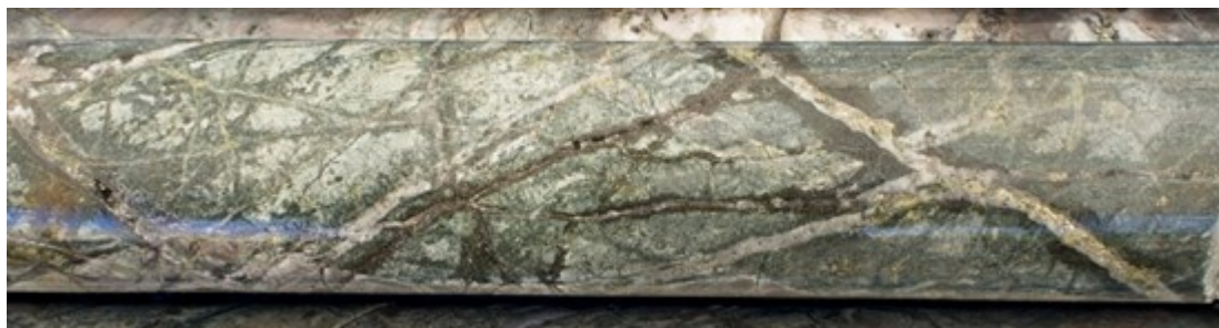
Image 1. Example of strongly veined and altered feldspathic arenite in ELID025 at 148.9 m from a 2 m long sample interval reporting 3.77% Cu, 0.009% Mo, and 31.6 g/t Ag . Chalcopyrite is concentrated along early quartz veinlets (A-type veins) and early sulfide veins associated with secondary biotite. The dark haloes around some veins is secondary biotite. Core is HQ diameter (63.5 mm).
