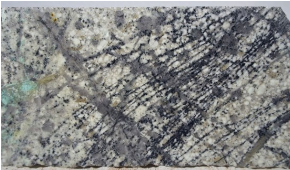
Figure 2. A specimen of drill core from drill hole FDC012 at 81.4 m within a sampled interval from 79.9 to 81.6 m reporting total Cu of 1.1%. Sulphuric acid leach (CuAS) was 0.14% Cu, sodium cyanide leach (CuCN) was 0.90% Cu, and four-acid leach (CuR) was 0.04%. This indicates most Cu is contained in the mineral chalcocite and a minor amount of Cu occurs as Cu oxide, which is the green mineral on the left side of the photograph. Chalcocite is the black mineral forming lines diagonally across the specimen and disseminated black points.
