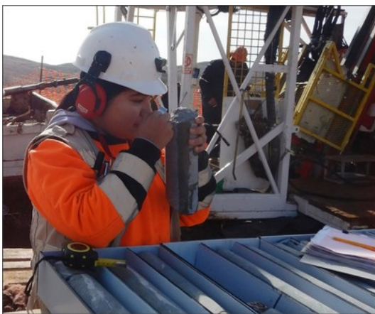
Figure 3: Zacatecas field geologist completing geotechnical logging of core at the Panuco North Vein drill site. (CNW Group/Zacatecas Silver Corp.)
