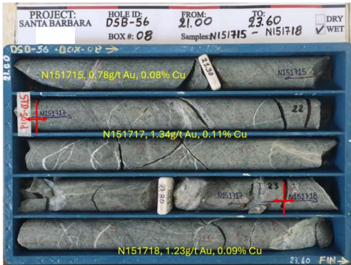
Figure 6: Core photo of DSB-56, Box 08, from 21m to 23.6m, mineralized diorite with quartz veining.
