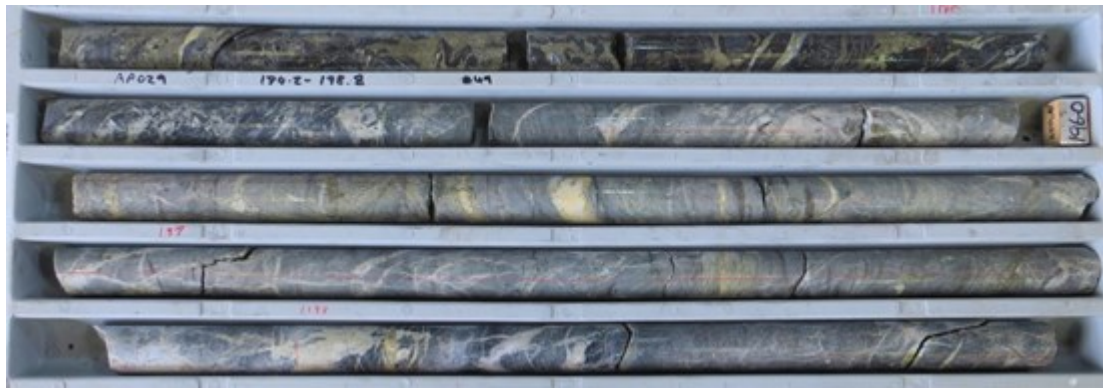
Figure 7. Photo of drill core from hole AP029 (194.2-198.8m), showing typical disseminated, blebby and vein style sulphide mineralization associated with silica-siderite alteration and veining.
