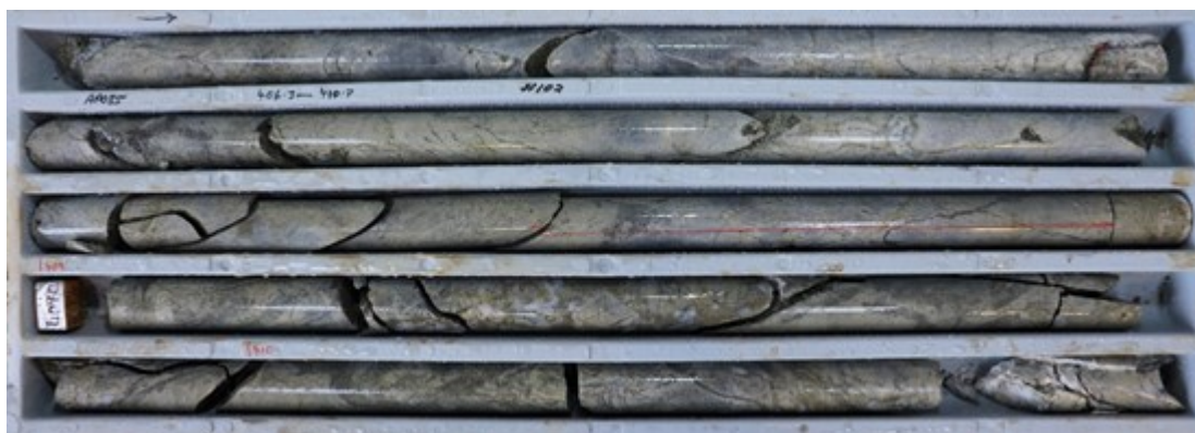
Figure 12. Photo of drill core from hole AP035 (406.3-410.7m), showing typical disseminated, blebby and vein style sulphide mineralization associated with silica-siderite alteration and veining. Assays pending.
