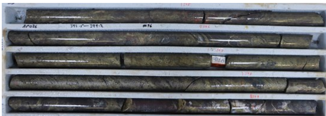
Figure 13. Photo of drill core from hole AP036 (394.5-399.2), showing chalcopyrite mineralized massive magnetite-pyrite-hematite-siderite rock. Assays pending.
