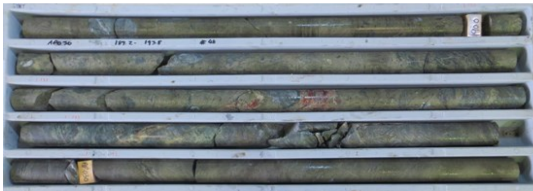
Figure 9. Photo drill core from hole AP030 (189.2-193.8m), part of the magnetite-pyrite-hematite-siderite hosted high-grade intercept, 10m @ 1.20% Cu from 185m.
