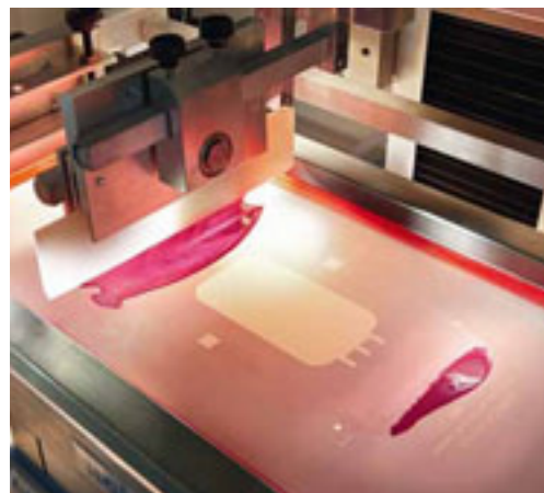
The layers of a functional film are applied individually by screen printing.
