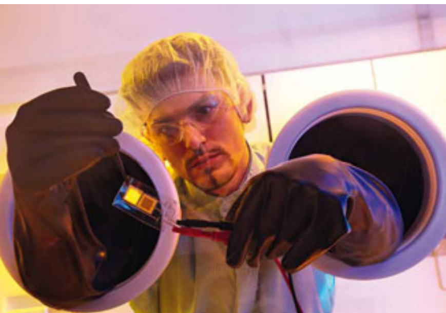
In the production of organic light-emitting diodes, Nicolas Degiorgio makes use of a nitrogen chamber free of oxygen and moisture.
