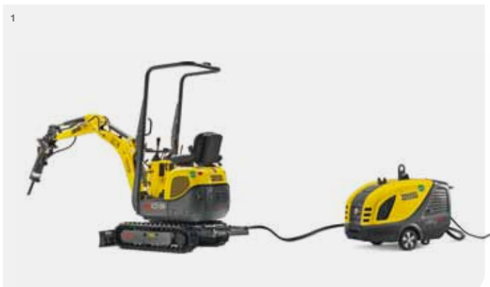
1 "dual power" The first series excavator from Wacker Neuson equipped with a zero-emission electric hydraulic motor (for zero emissions when working indoors, for example). The "plug & play" hydraulic power unit (HPU) can be easily connected and used instead of the diesel engine.
