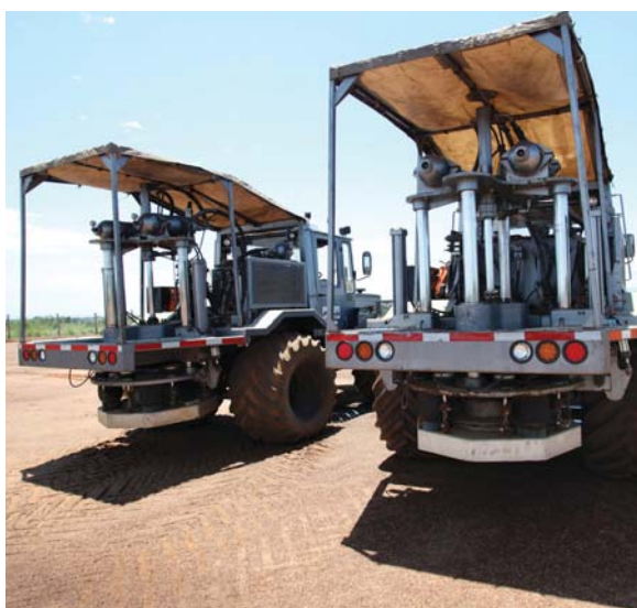
Accelerated weight drop units used in seismic acquisition, in EA 2, Uganda.
