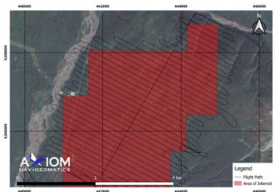
Figure 9.8: Flight Path Sample for the LiDAR Survey
