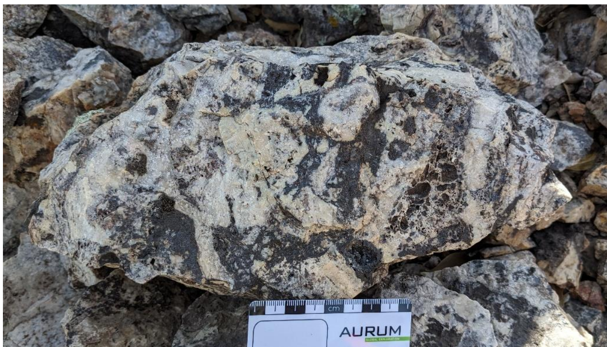
Figure 7-7: Brecciated Quartz Vein Containing a Matrix of Fe and Mn Oxides from the La Matilera Prospect - the Sample Contained 73.7 g/t Ag
