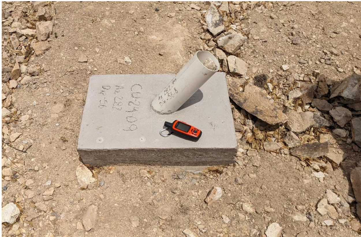
Figure 10-2: Cement Marker Denoting the Location of a Drill Hole Collar
