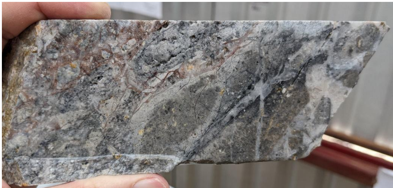
Figure 7-4: Drill Core Showing Brecciated and Silicified Rhyodacite Fragments (Right) Adjacent to a Silica-Flooded Quartz Vein
