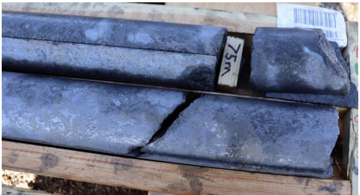
Figure 5: Photo highlighting the coarse flake graphite in NAG25-01.
