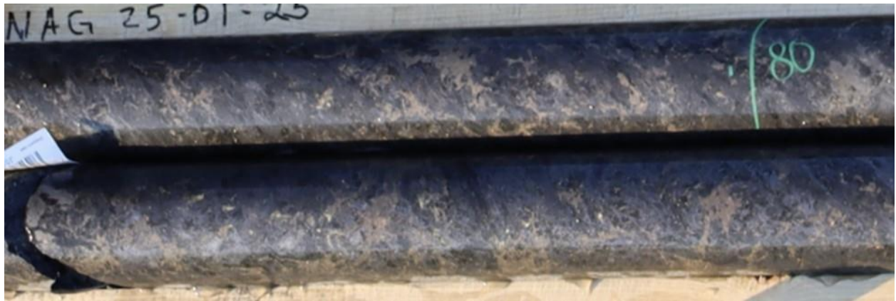
Figure 4: A close-up of the sulphide mineralization at the 80-81 metre interval.
