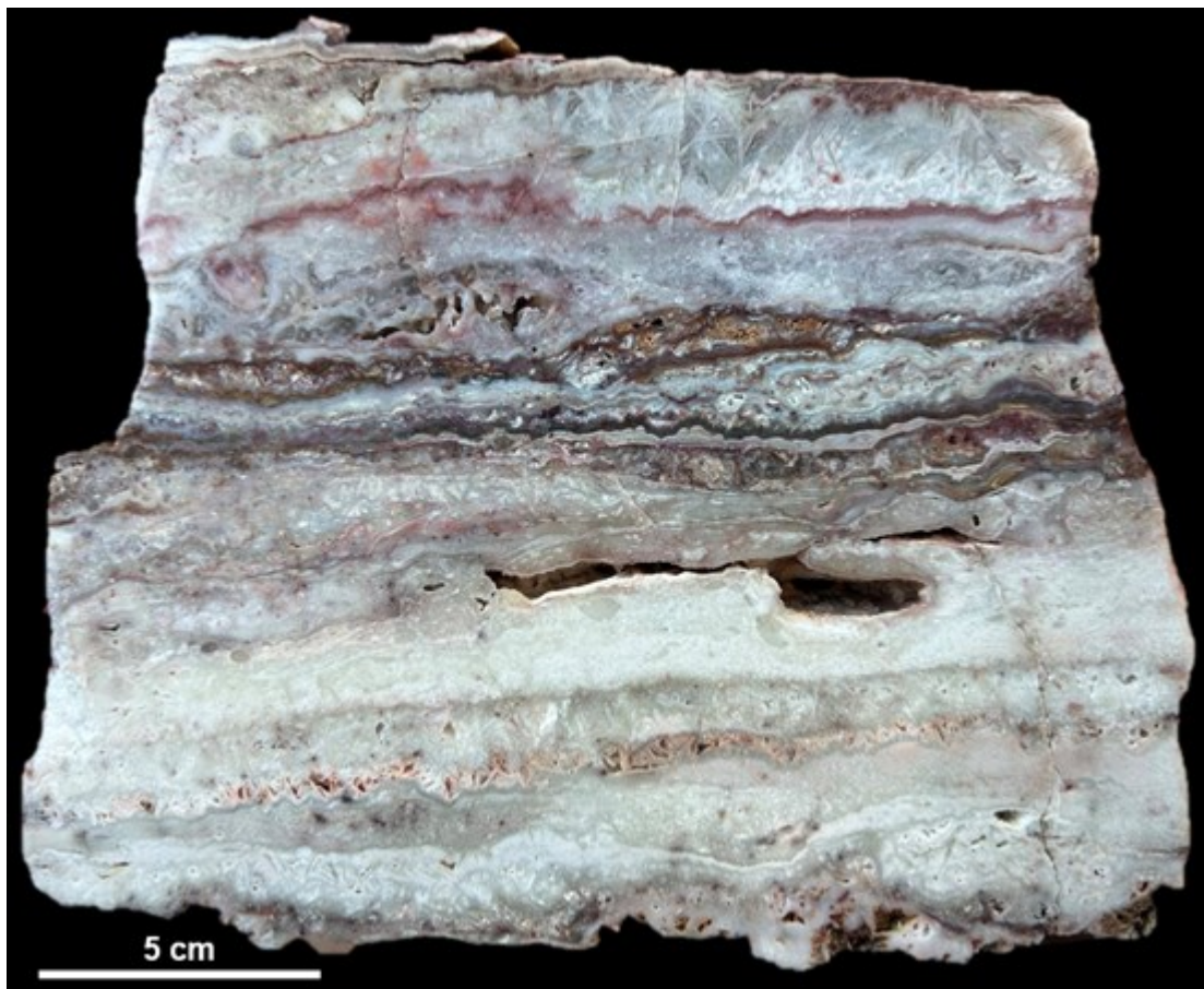
Figure 3: Vein material from outcropping vein at Table Mountain displaying crustiform-colloform banded chalcedony and fine-grained quartz textures with silicified bladed (platy) calcite, consistent with an upper-level low-sulphidation epithermal environment.
