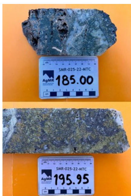
Figure 2: Close-up view of mineralized intervals of drill core; photo A: semi-massive sulphides, including abundant galena, silver sulphosalts, sphalerite, chalcopyrite, with quartz and rhodochrosite gangue minerals, Matacaballo vein hole SMR-25-22-MTC, 185.00 m depth; photo B: chalcopyrite-rich interval of massive sulphide vein segment, also showing galena, sphalerite, pyrite, Ayayay vein, hole SMR-25-22-MTC, 195.95 m depth. (CNW Group/Silver Mountain Resources Inc.)
