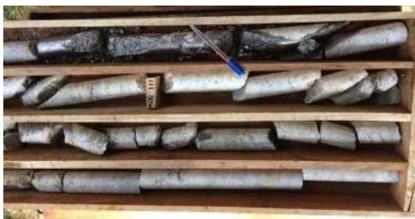
Picture No 22: Core box of drill hole DH003 showing in the first row the 60 cm long intersection of the graphite vein. The core shows fracturation at 30° core angle which are not reported in the drill log. The host rock is described as a garnet-biotite gneiss (source: Kithsiri Palandagama P. Geo., M.Sc., 04-2018).
