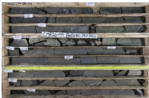
Figure 3: Copper-rich and zinc-rich massive sulphide mineralization from drill hole CMR26-199.[1]
