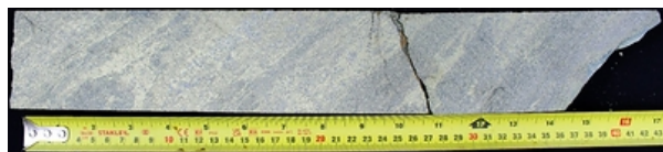
Figure 2: A higher copper grade section from CMR26-199 showing abundant chalcopyrite mineralization.[1]
