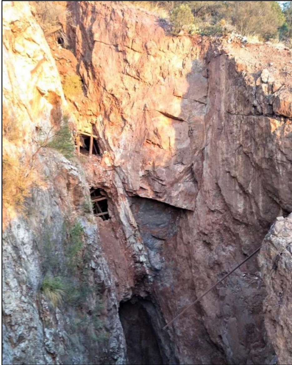
Figure 6-2: Underground Drifts Exposed in Surface Stope on Fanney Vein, Looking SE
