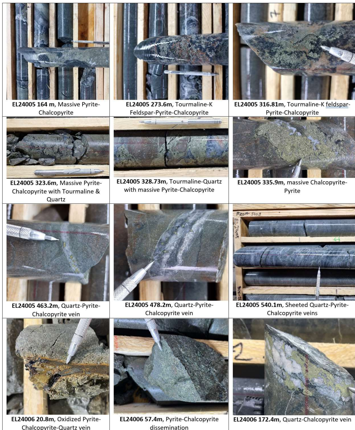
Figure 6. Drill core photos from holes EL24005 and EL24006 showing alteration, vein styles and mineralization.
