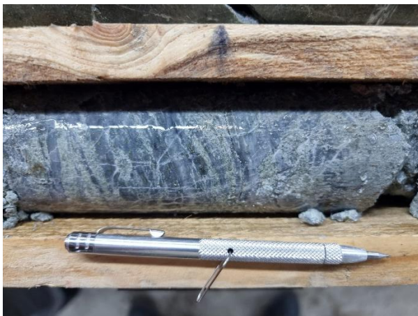
EL24005_536.9m Sheeted quartz-pyrite-chalcopyrite veins
