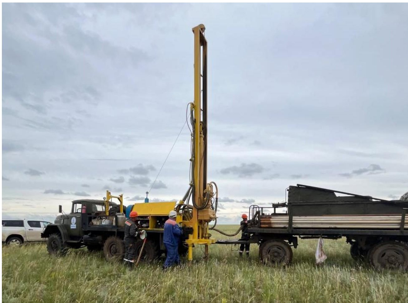
Figure 41: Burstroy KGC drill-rig.
