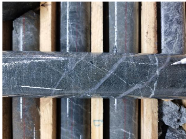
EL24005_533.0m Quartz-pyrite-chalcopyrite veins
