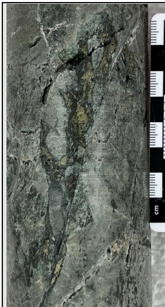
EL25012_54.0 m Disseminated chalcocite and pyrite
