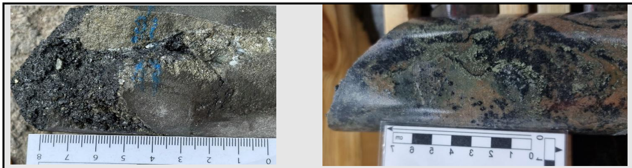
EL24016_60.6m Enargite, chalcopyrite and pyrite cementing diorite fragments
