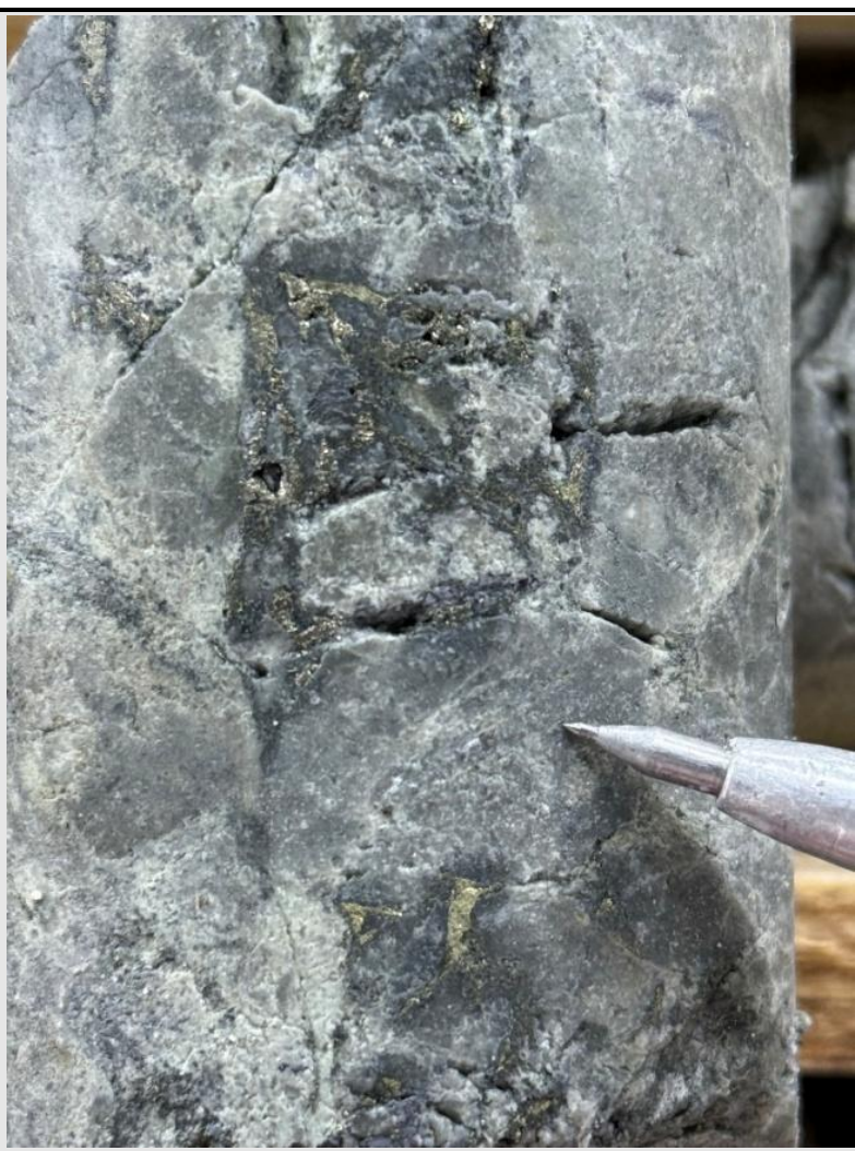
EL25012_187.5 m Chalcopyrite-pyrite-molybdenite patches in brecciated and silicified diorite
