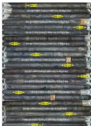
Figure 5. Core photos for DKD039 showing high-grade zone of 19.6 m grading 1.51% CuEq (1.30% Cu, 0.29g/t Au, 2.26g/t Ag) from 693.1 m within the broader high-grade zone 61.5m grading 1.03% CuEq (0.90% Cu, 0.18g/t Au) from 670.7 m. (CNW Group/Hot Chili Limited)
