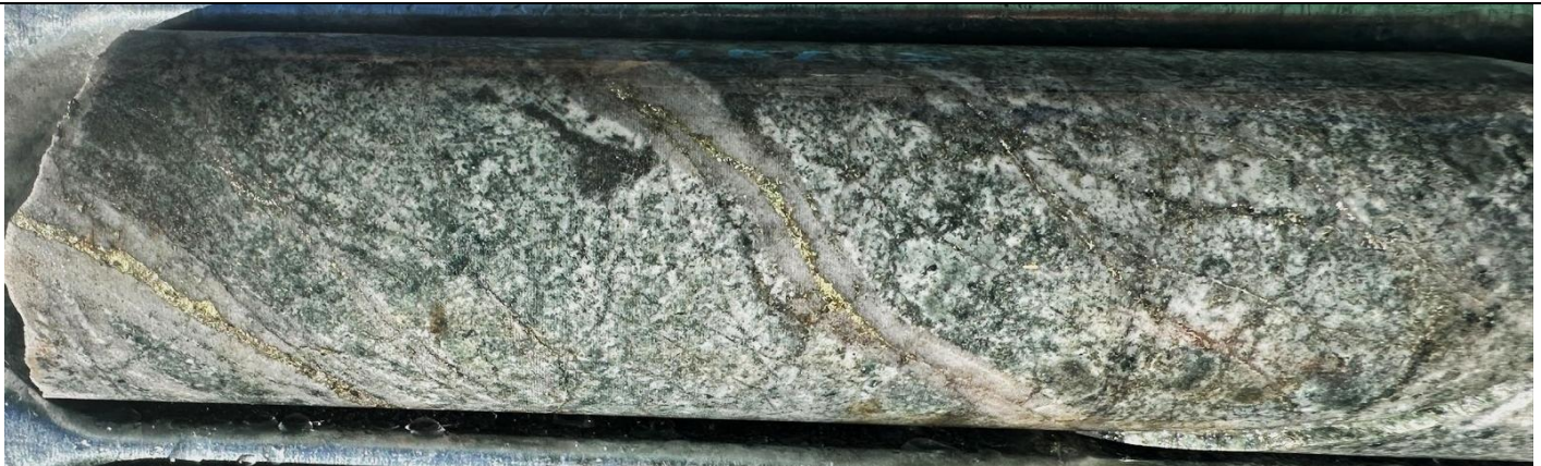
Core photo from DKD049 (541 m downhole) showing vein-hosted and disseminated chalcopyrite (2%) and pyrite (2.5%) mineralisation in strongly A-B veined tonalite host rock. Broad 180 m down-hole visual drill intersection represents a significant 175 m step-out to La Verde's high-grade core along its eastern flank, assay results expected May 2026 1
