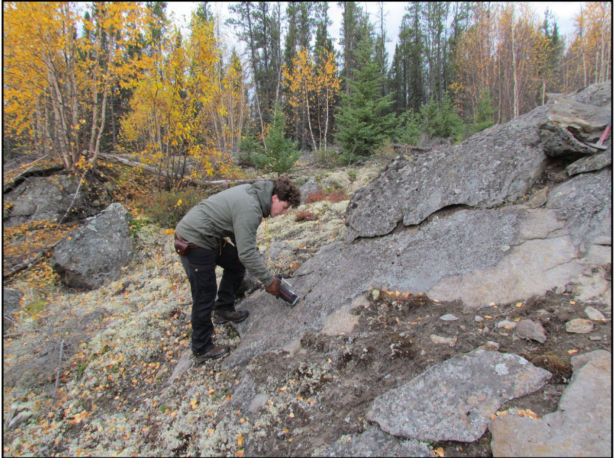
Figure 12-2: Troy Marfleet, QP, testing for radioactivity at the “D Zone” Outcrop
