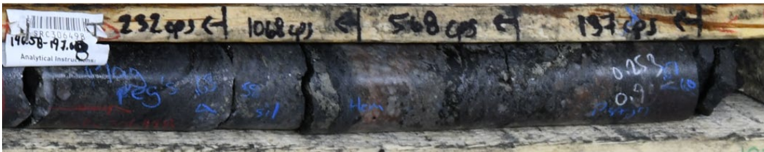
Figure 2. Drill section from drillhole FN24001 and drill core photo from anomalous interval which returned 378 ppm U 3 O 8 .
