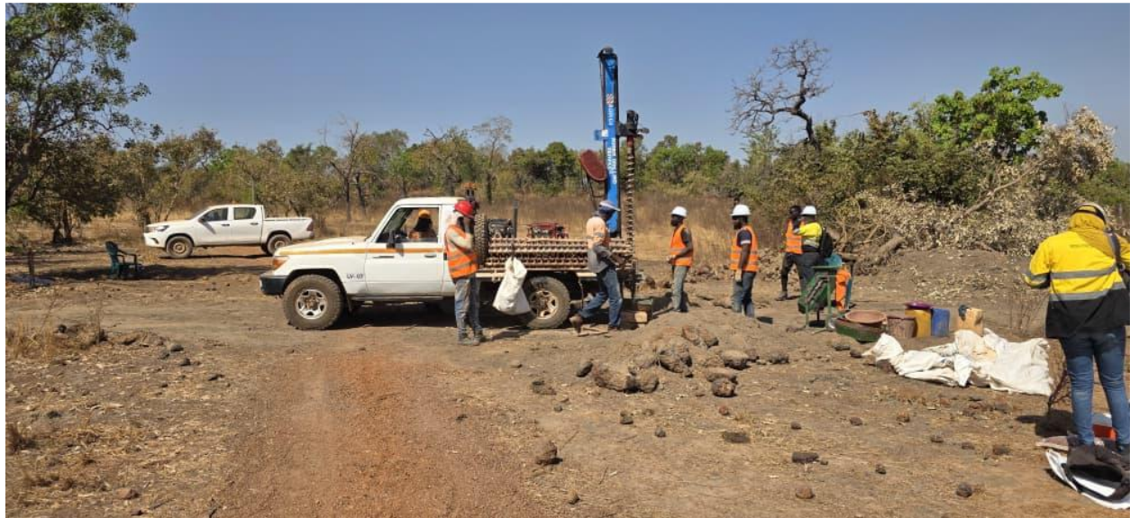
Figure 2: Power Auger tool, Systematically Sampling the Saprolite Underneath the Laterite Cover at Daina
